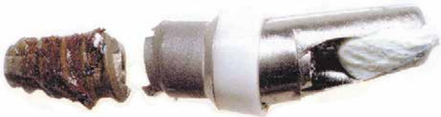
Sample after breaking – All breaks occurred at the same place on the implant body (at the beginning of intra-osseous thread)
