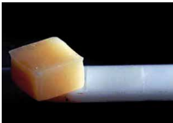
Yttria-Tetragonal Zirconia Polycrystal dental block
